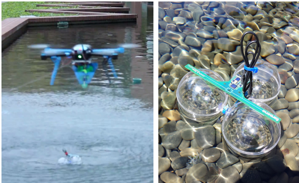
Fig. 11. Drone reading a sensorized tag to assess water quality. Drones could take sensor measurements in difficult to reach locations over water.
