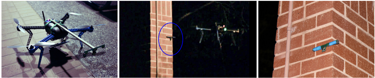
Fig. 10. Mobile robots could be used to affix sensors in hard-to-reach or difficult-to-service locations, such as retrofitting buildings, bridges, or treetop canopies with sensor tags. In this case, we outfitted a UAV with a boom arm tipped with an adhesive-backed sensor tag (left). Under RC control, the UAV deployed the tag and could return later to take measurements (middle and right).
