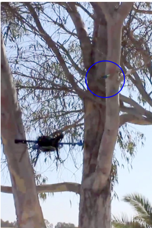
Fig. 13. Drone reading a sensorized tag in a tree. Drones could be used for forestry monitoring to read sensors in the forest canopy.
