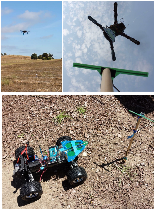
Fig. 1. Top Row: An unmanned aerial vehicle (a quadrotor drone) from 3D Robotics hovers above a Farsens Hydro tag mounted on a stick. The drone uses an attached UHF RFID reader to obtain direct soil moisture measurements from the tag. Bottom: An autonomous ground vehicle with a UHF RFID reader approaches a similar Farsens Hydro tag and obtains direct soil moisture measurements.
