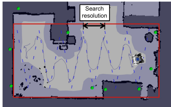
Fig. 4. The PR2 was commanded to perform sparse global RFID search with a 1.5 m resolution, constrained by the red rectangular search region. An overhead map of the home shows the robot-generated navigation waypoints (blue arrows), the robot's actual search path (blue line), tag positions (green circles), and navigation obstacles (purple regions).
