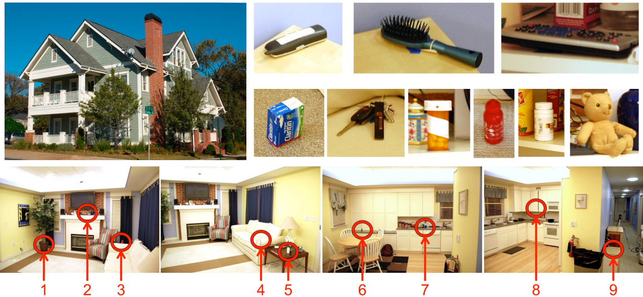
Fig. 6. Top Left: The Georgia Tech Aware Home where we tested our approach. Top Right: The nine tagged objects we used to evaluate our approach. From left-to-right: cordless phone, hair brush, TV remote, medication box, keys, medication bottle, water bottle, vitamin bottle, and teddy bear (toy). We tagged objects with Alien ALN-9640 Squiggle tags, with the exception of the TV remote and keys, which we tagged with Sontec metal-mount tags. Bottom: Photographs of the nine different test locations in the Aware Home’s kitchen, dining, and living rooms.
