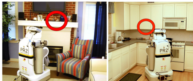
Fig. 1. Two final robot configurations after performing our UHF RFID search algorithm for a tagged object on a fireplace mantle and inside a kitchen cabinet. Object locations are denoted by red circles.
