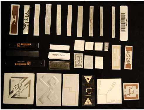
Fig. 2. EL-E’s in-hand reader has been demonstrated to work with numerous types / variants of UHF RFID tags, including the thirty-two different types of tags shown here.
