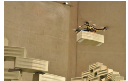
Figure 10. A quadrotor helps assemble a tower as part of an art project by ETH Zurich roboticists and architects. (Photo courtesy of Markus Waibel.)
