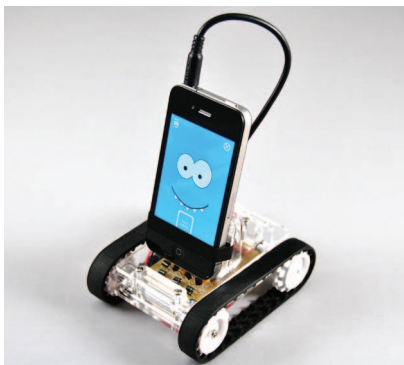
Figure 5. Romotive, a Seattle start-up, created a tracked mobile robot powered by a smartphone. (Photo courtesy of Romotive.)
