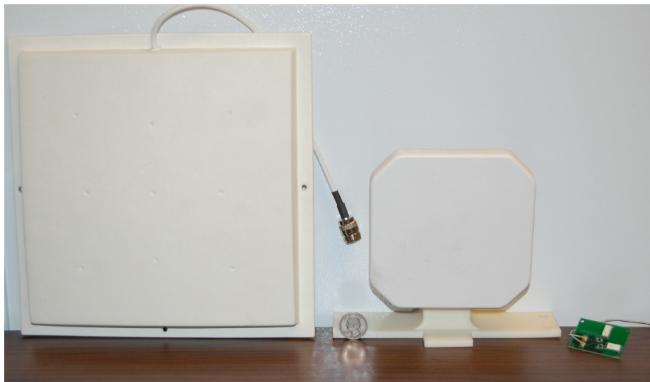
Figure 8: UHF RFID Antennas. From left-to-right: Laird Technologies S9028PC12NF long-range patch antenna, a quarter (US $0.25) for scale, Laird Technologies S9025P long-range patch antenna, and Johanson Technology (part number 0920AT50A080E) short-range ceramic microstrip antennas.
