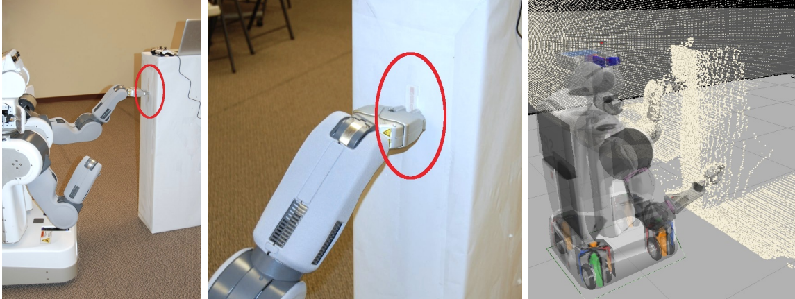
Figure 23: Using simultaneous localization and mapping (SLAM), we track the robot’s pose on a map (right). Using the forward kinematics of the robot’s arms, we can determine the pose of the tag in the map frame (left and middle).
