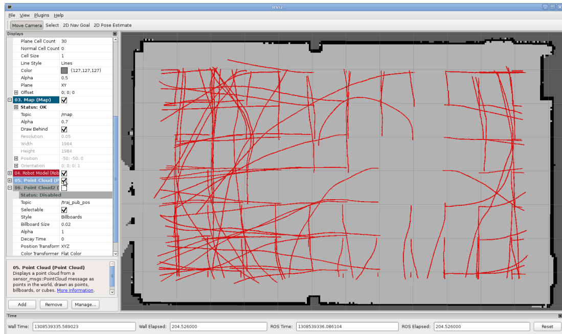
Figure 56: The PR2 robot uses its two shoulder-mounted RFID antennas to servo to the vertically-oriented RFID tag. These figures illustrate the robot’s trajectories for initial conditions that resulted in successful (top) and unsuccessful (bottom) approaches to the tag.
