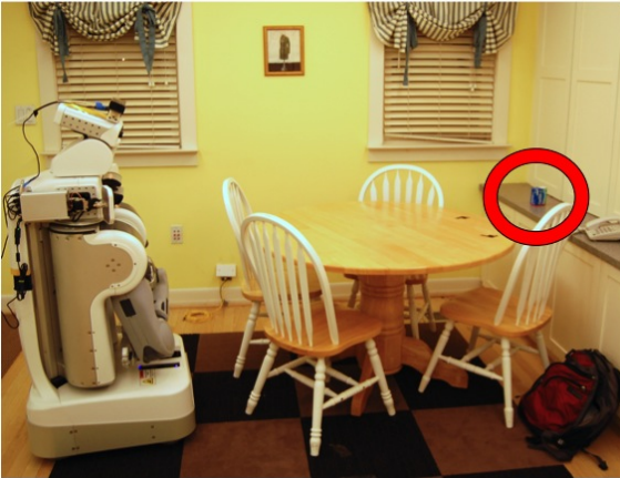
Figure 77: The results for RFID search with tagged objects at location 5. Top: The locations of positive and negative reads (grey and red, respectively) during RFID search (blue robot trajectory), the “best” location given by global search (orange), and the final location after servoing (teal). Bottom: A photograph of the PR2 post-servoing and a 3D point cloud captured by the PR2’s head-mounted Kinect showing the robot’s perspective.
