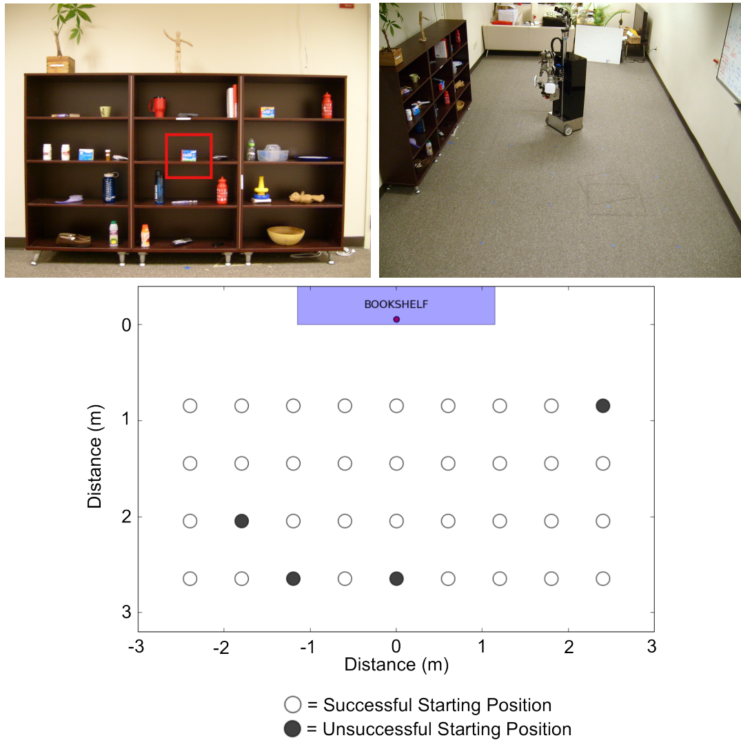
Figure 58: Top Row: In a large room (right), a bookshelf contains 37 tagged objects. EL-E has been tasked with approaching the tagged medication box, boxed in red (left). Bottom Row: The results of EL-E approaching the tagged object (red circle). White circles indicate success; black circles indicate failure.
