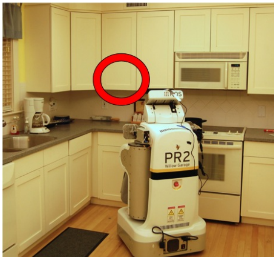
Figure 79: The results for RFID search with tagged objects at location 7. Top: The locations of positive and negative reads (grey and red, respectively) during RFID search (blue robot trajectory), the “best” location given by global search (orange), and the final location after servoing (teal). Bottom: A photograph of the PR2 post-servoing and a 3D point cloud captured by the PR2’s head-mounted Kinect showing the robot’s perspective.
