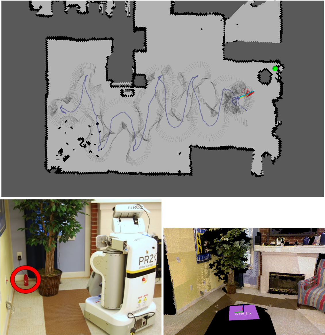
Figure 72: The results for RFID search with tagged objects at location 0. Top: The locations of positive and negative reads (grey and red, respectively) during RFID search (blue robot trajectory), the “best” location given by global search (orange), and the final location after servoing (teal). Bottom: A photograph of the PR2 post-servoing and a 3D point cloud captured by the PR2’s head-mounted Kinect showing the robot’s perspective.
