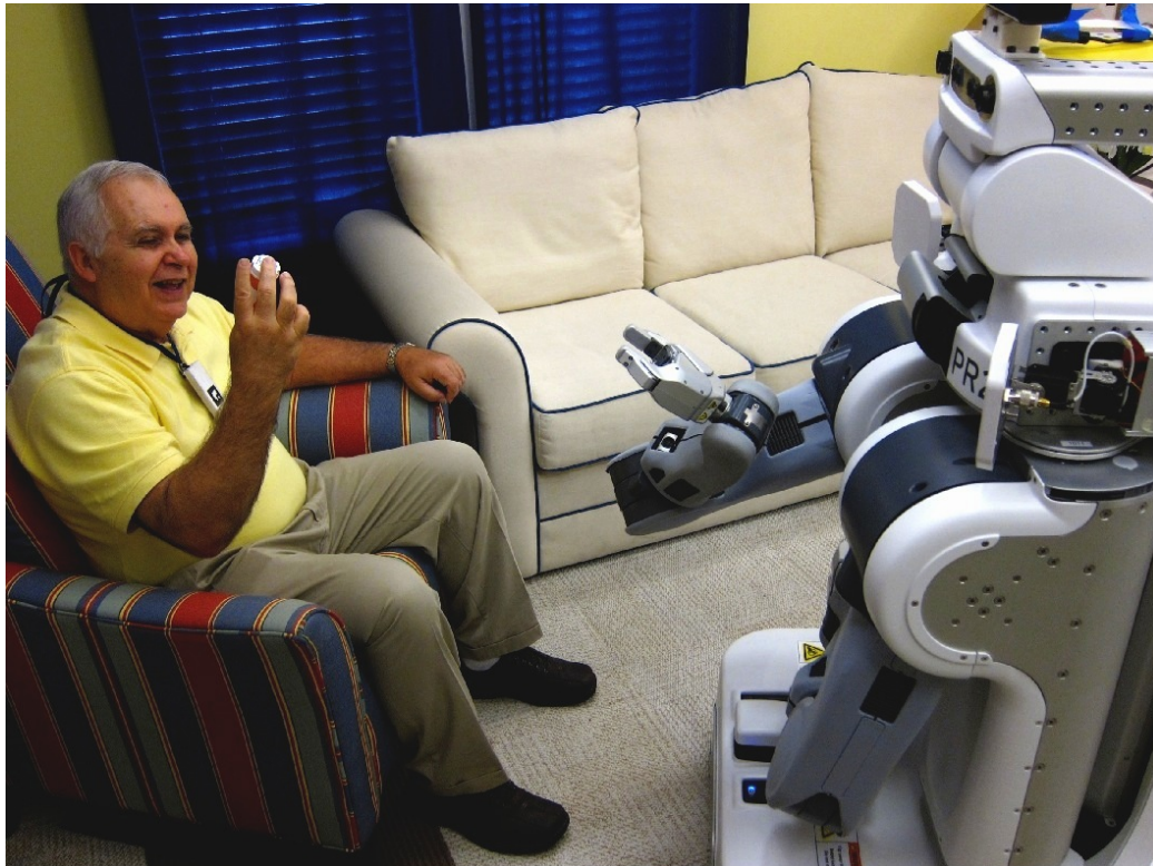
Figure 115: The Human Factors and Aging Lab at Georgia Tech is currently running user studies to understand how older adults perceive personal robots. UHF RFID medication delivery is one of the demonstrations and technologies being examined. In this demonstration (not actually part of the user study), the PR2 has successfully demonstrated UHF RFID medication delivery to an older adult seated in Georgia Tech's Aware Home. [Photo used with user permission.]
