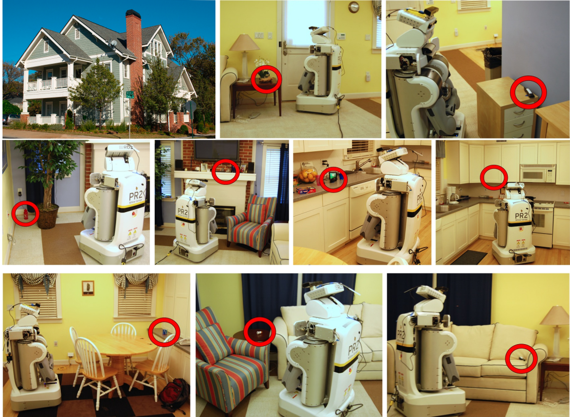
Figure 2: We tested our hybrid global-local RFID search algorithm in a real home environment (Georgia Tech’s Aware Home, top left). As shown in the photographs, the robot obtains positions near the desired tagged object(s) and oriented toward them for various locations inside the home. Details are available in Chapter 4.
