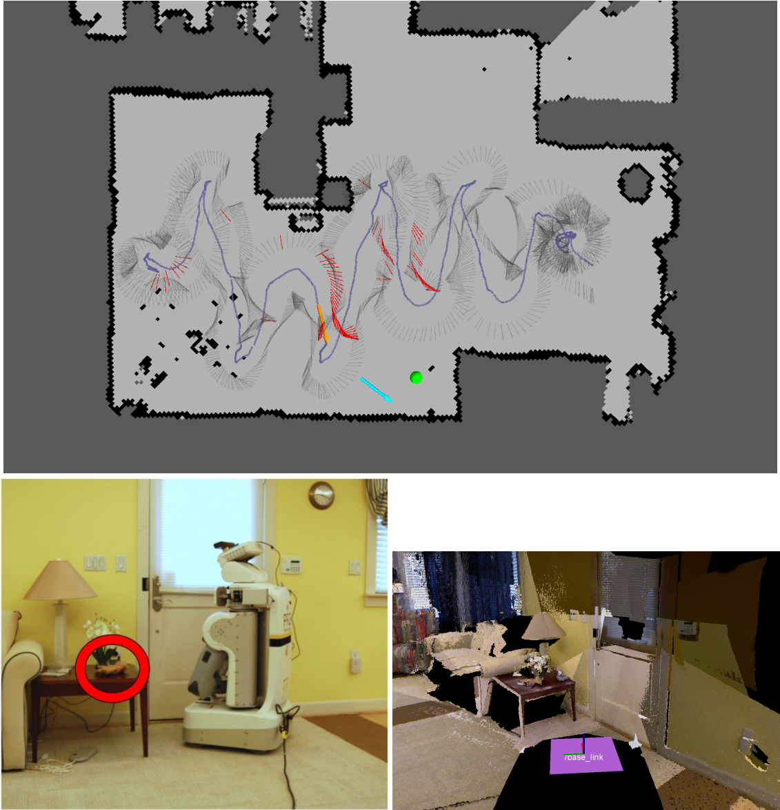
Figure 76: The results for RFID search with tagged objects at location 4. Top: The locations of positive and negative reads (grey and red, respectively) during RFID search (blue robot trajectory), the “best” location given by global search (orange), and the final location after servoing (teal). Bottom: A photograph of the PR2 post-servoing and a 3D point cloud captured by the PR2’s head-mounted Kinect showing the robot’s perspective.
