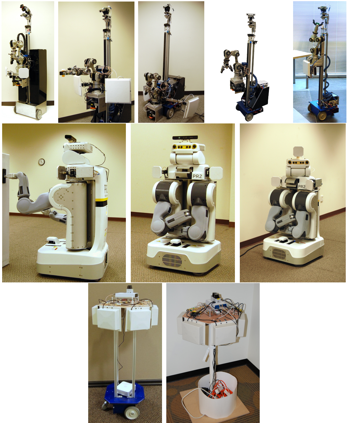
Figure 12: Over the course of performing our research, we used several different robots. The robots were in a continuous state of evolution. Here are some snapshots of the robots: EL-E (top), PR2 (middle), test rigs (bottom).
