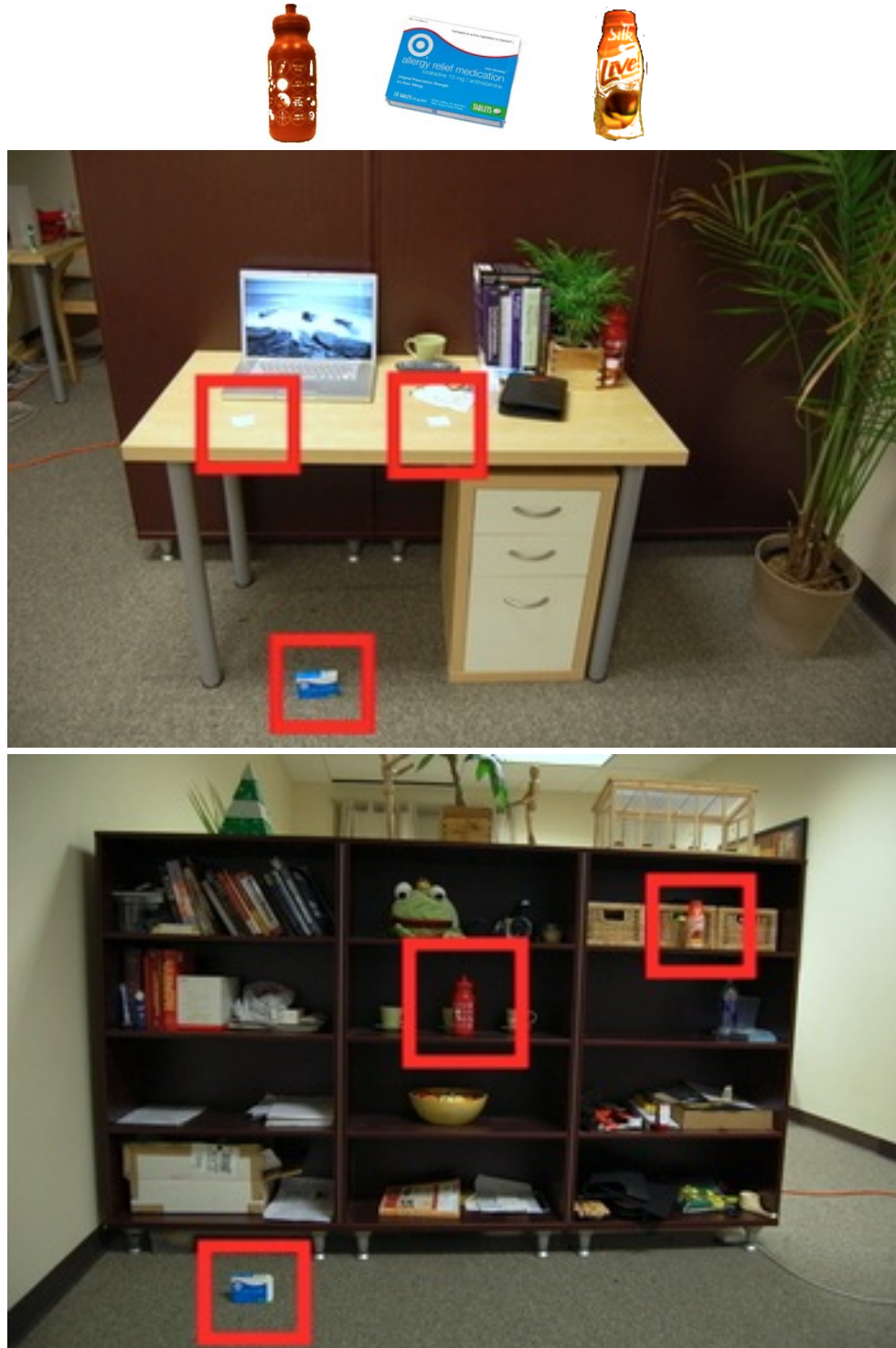
Figure 110: The two scenes for sensor fusion experimentation. The sole failure occurred when the orange disposable bottle was placed in the upper-right location in the bottom scene.
