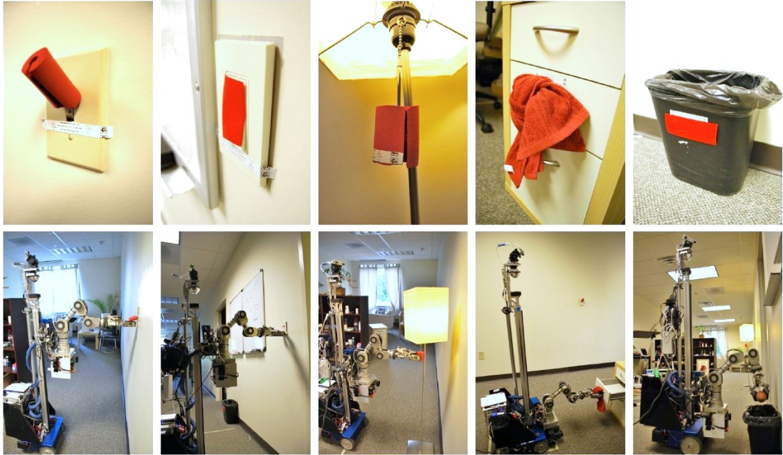
Figure 101: Top Row: PPS-tags affixed to a flip-type light switch, a rocker-type light switch, a pull-chain lamp, a cabinet drawer, and a trashcan. Bottom Row: EL-E interacting with each of these PPS-tags.
