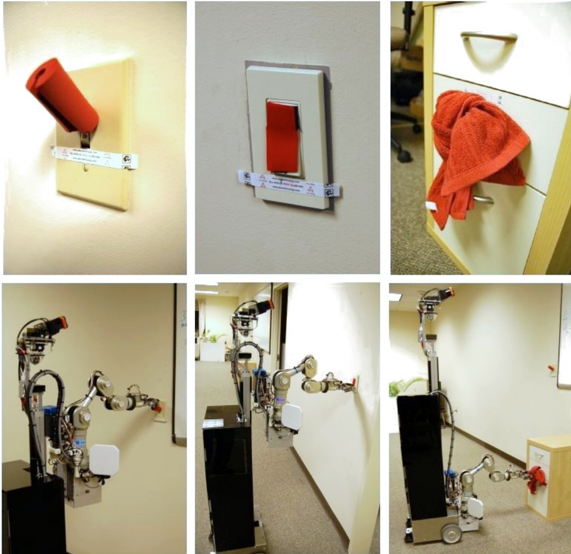
Figure 92: Top Row: PPS-tags affixed to a flip-type light switch, a rocker-type light switch, and a cabinet drawer. Bottom Row: EL-E interacting with each of the PPS-tags.
