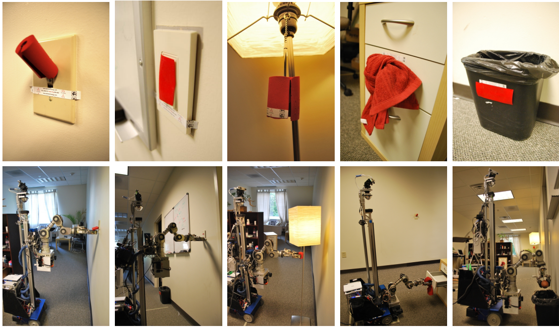
Fig. 2. Top : PPS-tags affixed to (from left to right): flip-type light switch, ADA-compliant rocker-type light switch, lamp pull chain, cabinet drawer, and trashcan. Bottom : EL-E manipulating the corresponding PPS-tags.
