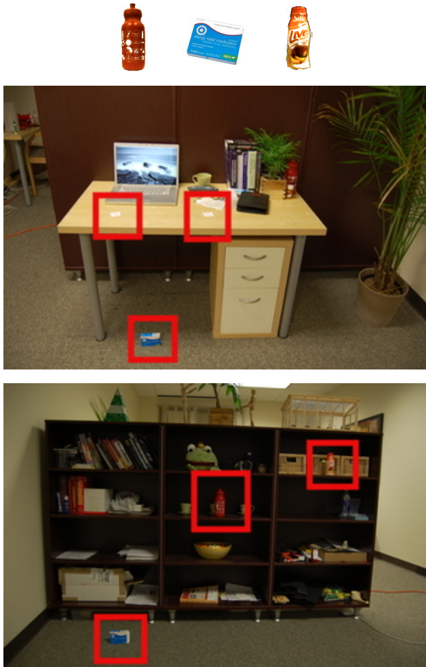
Fig. 9. Three test objects: red water bottle, blue medication box, and orange disposable bottle (top). The two scenes and their three associated object placement locations are indicated. The sole failure occurred when the orange disposable bottle was placed in the upper-right placement location in the bottom scene.
