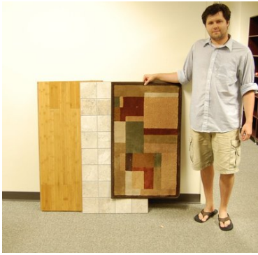
Fig. 6. Four common floor types used in the experiments: Wood floor, short pile carpet, tile floor, and medium pile carpet
