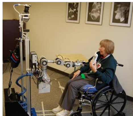
Fig. 1. The autonomous mobile manipulator EL-E (pronounced “Ellie”) delivering a cordless phone to an ALS patient – photo used with patient permission and IRB approval.
