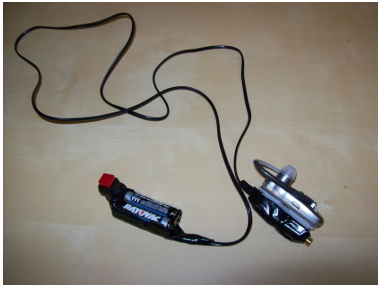
Figure 9: Ear-mounted laser pointer and a wired button
