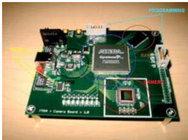
Figure 1: The produced PCB with FPGA, USB, memory and image sensor.
